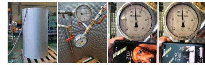
[Water Pressure Test] 24.1 bar, 30 min hold. (Same before and after thermal cycle)
