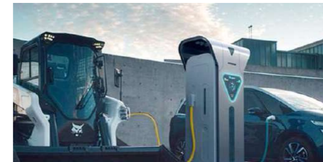
* A concept image of charging a fully electric loader and hydrogen car through Tri-gen, which generates hydrogen, electricity, and heat
