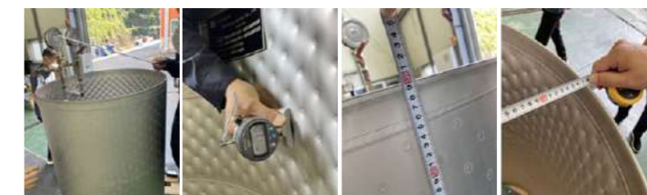
[Visual test for deformation of welding] Visual and Form3-based dimension inspection of welded parts (Measured after the thermal cycle to compare spec compliance and data)
